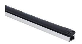
ASO Safety Solutions safety contact edge, 15 x 10mm, 2ft length, pigtail, 8.2ft/2.5m cable length. Aluminum mounting rail included. Preassembled with 8.2k ohm resistor for 2-wire installation.
