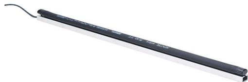
ASO Safety Solutions safety contact edge, 15 x 10mm, 1.5ft length, pigtail, 8.2ft/2.5m cable length. Aluminum mounting rail included. Preassembled with 8.2k ohm resistor for 2-wire installation.
