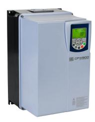
WEG Electric CFW500 series AC high-performance drive, NEMA 4X, 460 VAC, 20hp with 3-phase input, SVC, V/Hz, VVW, FOC or torque mode, B frame, RS-485, integrated dynamic braking. Optional communication and STO modules available.
