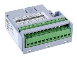
WEG Electric CFW500 series relay/analog combo module, Analog Input: 1-channel, current/voltage, Analog Output: 1-channel, current/voltage, Discrete Input: 5-point, sinking/sourcing, Discrete Output: 5-point, relay, (3) Form A (SPST) relays, (1) Form C (SPDT) relay.
