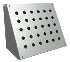
Hammond pushbutton consolet, 30 holes, 22mm, NEMA 12/13, 13 x 16 x 10in (HxWxD), desktop or pedestal mount, carbon steel, ANSI 61 gray, powder coat finish, hinged screw cover.
