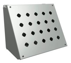
Hammond pushbutton consolet, 20 holes, 22mm, NEMA 12/13, 11 x 13 x 9in (HxWxD), desktop or pedestal mount, carbon steel, ANSI 61 gray, powder coat finish, hinged screw cover.
