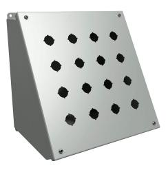
Hammond pushbutton consolet, 16 holes, 22mm, NEMA 12/13,  $11 \times 11 \times 9$ in (HxWxD), desktop or pedestal mount, carbon steel, ANSI 61 gray, powder coat finish, hinged screw cover.
