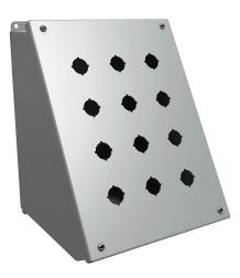
Hammond pushbutton consolet, 12 holes, 22mm, NEMA 12/13, 11 x 9 x 9in (HxWxD), desktop or pedestal mount, carbon steel, ANSI 61 gray, powder coat finish, hinged screw cover.
