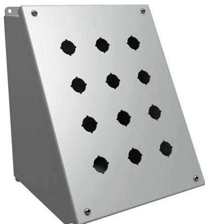
Hammond pushbutton console, 12 holes, 22mm, NEMA 12/13, 11 x 9 x 9in (HxWxD), desktop or pedestal mount, carbon steel, ANSI 61 gray, powder coat finish, hinged screw cover.
