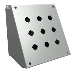
Hammond pushbutton consolet, 9 holes, 22mm, NEMA 12/13, 9 x 9 x 8in (HxWxD), desktop or pedestal mount, carbon steel, ANSI 61 gray, powder coat finish, hinged screw cover.
