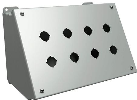
Hammond pushbutton console, 8 holes, 22mm, NEMA 12/13, 7 x 11 x 7in (HxWxD), desktop or pedestal mount, carbon steel, ANSI 61 gray, powder coat finish, hinged screw cover.
