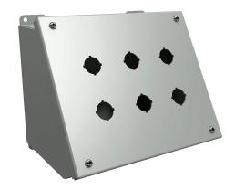
Hammond pushbutton consolet, 6 holes, 22mm, NEMA 12/13, 7 x 9 x 7in (HxWxD), desktop or pedestal mount, carbon steel, ANSI 61 gray, powder coat finish, hinged screw cover.
