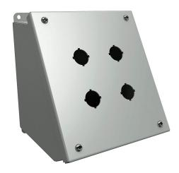
Hammond pushbutton consolet, 4 holes, 22mm, NEMA 12/13, 7 x 7 x 7in (HxWxD), desktop or pedestal mount, carbon steel, ANSI 61 gray, powder coat finish, hinged screw cover.
