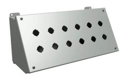
Hammond pushbutton consolet, 12 holes, 22mm, NEMA 12/13, 7 x 16 x 7in (HxWxD), desktop or pedestal mount, carbon steel, ANSI 61 gray, powder coat finish, hinged screw cover.
