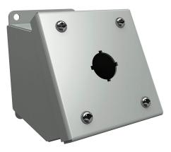
Hammond pushbutton consolet, 1 hole, 22mm, NEMA 12/13, 4 x 4 x 5in (HxWxD), desktop or pedestal mount, carbon steel, ANSI 61 gray, powder coat finish, screw cover.
