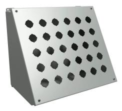
Hammond pushbutton consolet, 30 holes, 30mm, NEMA 12/13, 13 x 16 x 10in (HxWxD), desktop or pedestal mount, carbon steel, ANSI 61 gray, powder coat finish, hinged screw cover.
