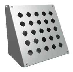
Hammond pushbutton consolet, 25 holes, 30mm, NEMA 12/13, 13 x 13 x 10in (HxWxD), desktop or pedestal mount, carbon steel, ANSI 61 gray, powder coat finish, hinged screw cover.
