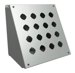
Hammond pushbutton consolet, 16 holes, 30mm, NEMA 12/13,  $11 \times 11 \times 9$ in (HxWxD), desktop or pedestal mount, carbon steel, ANSI 61 gray, powder coat finish, hinged screw cover.
