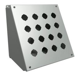
Hammond pushbutton consolet, 16 holes, 30mm, NEMA 12/13, 11 x 11 x 9in (HxWxD), desktop or pedestal mount, carbon steel, ANSI 61 gray, powder coat finish, hinged screw cover.
