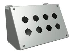
Hammond pushbutton consolet, 8 holes, 30mm, NEMA 12/13, 7 x 11 x 7in (HxWxD), desktop or pedestal mount, carbon steel, ANSI 61 gray, powder coat finish, hinged screw cover.
