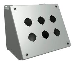
Hammond pushbutton consolet, 6 holes, 30mm, NEMA 12/13, 7 x 9 x 7in (HxWxD), desktop or pedestal mount, carbon steel, ANSI 61 gray, powder coat finish, hinged screw cover.
