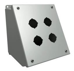
Hammond pushbutton consolet, 4 holes, 30mm, NEMA 12/13, 7 x 7 x 7in (HxWxD), desktop or pedestal mount, carbon steel, ANSI 61 gray, powder coat finish, hinged screw cover.
