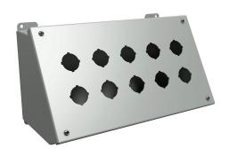
Hammond pushbutton consolet, 10 holes, 30mm, NEMA 12/13, 7 x 13 x 7in (HxWxD), desktop or pedestal mount, carbon steel, ANSI 61 gray, powder coat finish, hinged screw cover.
