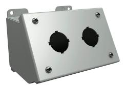
Hammond pushbutton consolet, 2 holes, 30mm, NEMA 12/13, 4 x 6 x 5in (HxWxD), desktop or pedestal mount, carbon steel, ANSI 61 gray, powder coat finish, screw cover.
