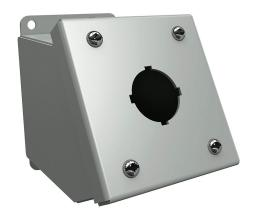
Hammond pushbutton consolet, 1 hole, 30mm, NEMA 12/13, 4 x 4 x 5in (HxWxD), desktop or pedestal mount, carbon steel, ANSI 61 gray, powder coat finish, screw cover.
