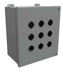
Hammond pushbutton enclosure, 9 holes, 30mm, NEMA 12, 11  $\times$  10  $\times$  6in (HxWxD), wall mount, carbon steel, ANSI 61 gray, powder coat finish, hinged screw cover.
