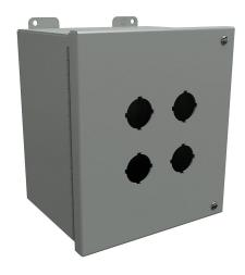
Hammond pushbutton enclosure, 4 holes, 30mm, NEMA 12, 9  $\times$  8  $\times$  6 in (HxWxD), wall mount, carbon steel, ANSI 61 gray, powder coat finish, hinged screw cover.
