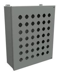
Hammond pushbutton enclosure, 42 holes, 30mm, NEMA 12, 20  $\times$  17  $\times$  6in (HxWxD), wall mount, carbon steel, ANSI 61 gray, powder coat finish, hinged screw cover.
