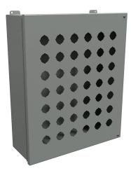
Hammond pushbutton enclosure, 42 holes, 30mm, NEMA 12, 20 x 17 x 6in (HxWxD), wall mount, carbon steel, ANSI 61 gray, powder coat finish, hinged screw cover.
