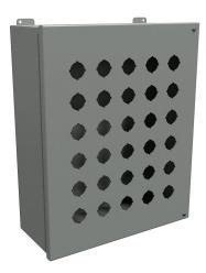
Hammond pushbutton enclosure, 30 holes, 30mm, NEMA 12, 18 x 14 x 6in (HxWxD), wall mount, carbon steel, ANSI 61 gray, powder coat finish, hinged screw cover.
