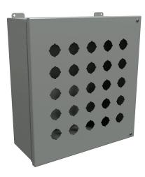
Hammond pushbutton enclosure, 25 holes, 30mm, NEMA 12, 15 x 14 x 6in (HxWxD), wall mount, carbon steel, ANSI 61 gray, powder coat finish, hinged screw cover.
