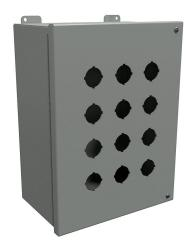
Hammond pushbutton enclosure, 12 holes, 30mm, NEMA 12, 13 x 10 x 6in (HxWxD), wall mount, carbon steel, ANSI 61 gray, powder coat finish, hinged screw cover.
