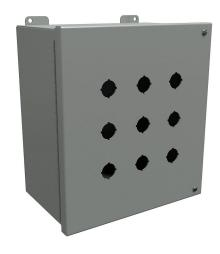
Hammond pushbutton enclosure, 9 holes, 22mm, NEMA 12, 11  $\times$  10  $\times$  6in (HxWxD), wall mount, carbon steel, ANSI 61 gray, powder coat finish, hinged screw cover.
