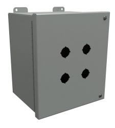
Hammond pushbutton enclosure, 4 holes, 22mm, NEMA 12, 9  $\times$  8  $\times$  6in (HxWxD), wall mount, carbon steel, ANSI 61 gray, powder coat finish, hinged screw cover.
