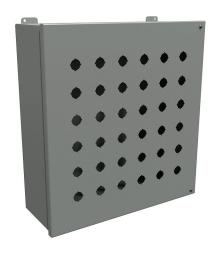
Hammond pushbutton enclosure, 36 holes, 22mm, NEMA 12, 18  $\times$  17  $\times$  6in (HxWxD), wall mount, carbon steel, ANSI 61 gray, powder coat finish, hinged screw cover.
