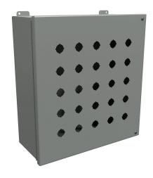
Hammond pushbutton enclosure, 25 holes, 22mm, NEMA 12, 15  $\times$  14  $\times$  6in (HxWxD), wall mount, carbon steel, ANSI 61 gray, powder coat finish, hinged screw cover.
