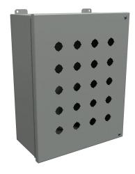
Hammond pushbutton enclosure, 20 holes, 22mm, NEMA 12, 15  $\times$  12  $\times$  6in (HxWxD), wall mount, carbon steel, ANSI 61 gray, powder coat finish, hinged screw cover.
