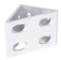
FATH gusseted inside corner bracket, silver, 90-degree, 8 holes, anodized aluminum, slot size 10. For use with all 45mm and 90mm profile T-slotted rails. Manufacturer part number: 093W8901N10.
