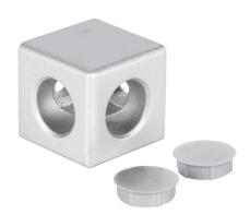
FATH 2D cube connector, silver, 45 x 45 x 45mm, die-cast aluminum, slot size 10. For use with all 45mm and 90mm profile T-slotted rails. (2) plastic cover caps included. Manufacturer part number: 093WW453N10.
