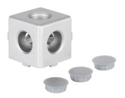
FATH 3D cube connector, silver,  $1.5 \times 1.5 \times 1.5$ in, die-cast aluminum, slot size 8. For use with  $1.5 \times 1.5$ in profile T-slotted rails. (3) plastic cover caps included. Manufacturer part number: 093WW382N08.
