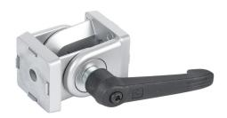
FATH pivot joint with locking handle, silver, 178-degree adjustable, 2 holes, die-cast zinc, slot size 8. For use with all 1.5in and 3in profile T-slotted rails. Manufacturer part number: 093GF38AN08.
