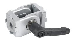
FATH pivot joint with locking handle, silver, 178-degree adjustable, 2 holes, die-cast zinc, slot size 6. For use with all 1in and 2in profile T-slotted rails. Manufacturer part number: 093GF25AN06.
