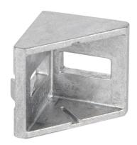
FATH angle bracket, silver, 90-degree, 2 holes, die-cast aluminum, slot size 8. For use with all 1.5in and 3in profile T-slotted rails. Manufacturer part number: 093W404N08.
