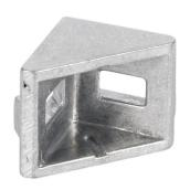
FATH angle bracket, silver, 90-degree, 2 holes, die-cast aluminum, slot size 6. For use with all 1in and 2in profile T-slotted rails. Manufacturer part number: 093W203N06.
