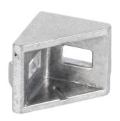
FATH angle bracket, silver, 90-degree, 2 holes, die-cast aluminum, slot size 6. Package of 10. For use with all 1in and 2in profile T-slotted rails. Manufacturer part number: 093W203N06.
