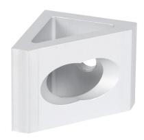
FATH gusseted inside corner bracket, silver, 90-degree, 2 holes, anodized aluminum, slot size 10. For use with all 45mm and 90mm profile T-slotted rails. Manufacturer part number: 093W8421N10.
