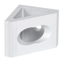
FATH gusseted inside corner bracket, silver, 90-degree, 2 holes, anodized aluminum, slot size 10. For use with all 45mm and 90mm profile T-slotted rails. Manufacturer part number: 093W8421N10.
