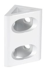
FATH wide gusseted inside corner bracket, silver, 90-degree, 4 holes, anodized aluminum, slot size 8. For use with 1.5 x 3in and 3 x 3in profile T-slotted rails. Manufacturer part number: 093WD8384N08.
