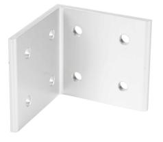
FATH inside corner bracket, silver, 90-degree, 8 holes, anodized aluminum, slot size 10. For use with all 45mm and 90mm profile T-slotted rails. Manufacturer part number: 093WD9090.
