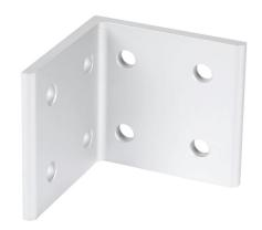
FATH inside corner bracket, silver, 90-degree, 8 holes, anodized aluminum, slot size 8. For use with all 1.5in and 3in profile T-slotted rails. Manufacturer part number: 093WD7676.
