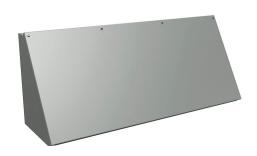
Hammond operator consolet, NEMA 12/13, 14 x 36 x 11in (HxWxD), desktop or pedestal mount, carbon steel, ANSI 61 gray, powder coat finish, screw cover.
