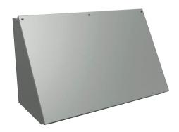
Hammond operator consolet, NEMA 12/13, 14 x 24 x 11in (HxWxD), desktop or pedestal mount, carbon steel, ANSI 61 gray, powder coat finish, screw cover.
