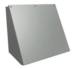
Hammond operator consolet, NEMA 12/13, 14 x 16 x 11in (HxWxD), desktop or pedestal mount, carbon steel, ANSI 61 gray, powder coat finish, screw cover.
