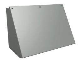
Hammond operator consolet, NEMA 12/13, 11 x 16 x 9in (HxWxD), desktop or pedestal mount, carbon steel, ANSI 61 gray, powder coat finish, screw cover.
